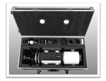
**A.** Upon delivery, and when not used, the telescope and its accessories are inside the aluminum padded case. Unpack the telescope and assemble it to your mount using the included D (Losmandy style) dovetail bar. Please refer to your mount manual to properly install the telescope.
