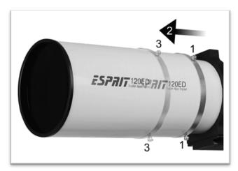
**B**. To extend the dew cap unscrew the two screws on the aluminum ring (1), then gently pull the dew cap forward (2). When in position, tighten the two screws to ensure the dew cap stays in position (3).
